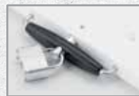
Trolling motor attaches to top of bracket. Bracket locks in over top of deck-mounted center puck.
